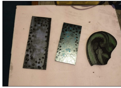
Above and left: Another transept window had three broken pieces. They were removed, sent to Iowa, reproduced and returned for installation. Thank you FedEx!
