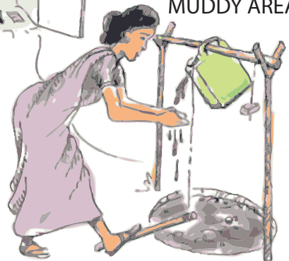
8. MAKE GRAVEL BASIN BETWEEN STICKS TO PREVENT MUDDY AREA
