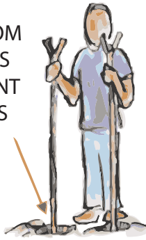
2. PLACE THE FORKED STICKS, ENSURE THEY ARE LEVEL
